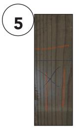
Use a measuring tape to create marks on each leg at 12" where the leg braces will be attached.
